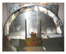
A 3-D crate imager based on a scanning laser range finder. The diameter of the scan arc is 50 cm.
