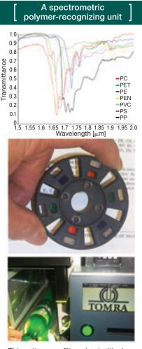
This unit uses a filter wheel with six polymer pieces as the spectrally discriminating element. (Top) Representative spectra of various polymer materials between 1.5 and 1.8 µm (characteristic spectral range of many collectable polymers). (Center) The filter wheel itself (Bottom) Entrance area of a reverse vending machine with the material detector.
