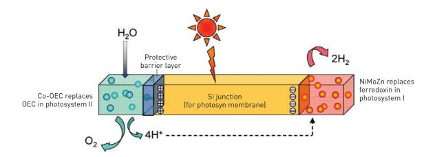
The structure of an artificial leaf produced by researcher Daniel Nocera's team features a silicon junction that captures photons. The cobalt-based oxygen evolving complex (Co-OEC) and a nickel, molybdenum and zinc alloy (NiMoZn) perform the watersplitting function and transport the captured energy into storage.
