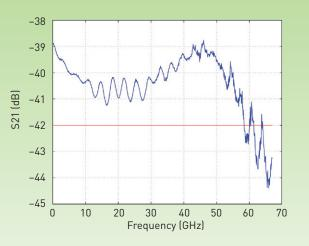
(Left) A high-speed photodetector fabricated in the OpSIS-IME platform with an inductor for gain-peaking bandwidth enhancement. (Right) The device has 57 GHz bandwidth.
