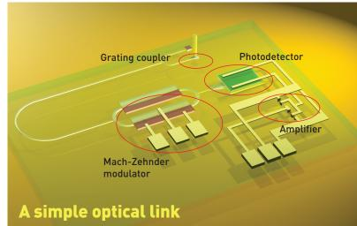
Link consists of a grating coupler, modulator, detector and amplifier.
