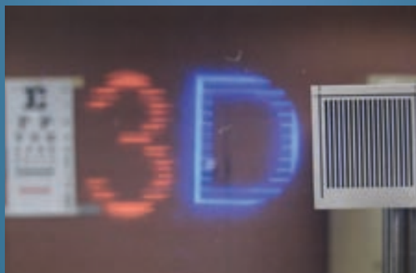
Effects of focusing the camera on the grating target 30 centimeters away.
