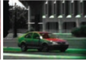
Color fusion image from a polarimeter based on polarization gratings, showing angle and degree of linear polarization.
