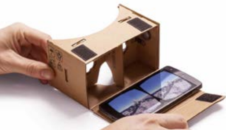
Google Cardboard is a simple head-mounted box with focusing lenses. The user's smartphone acts as both computer and display, serving up a stereo pair of images to create a 3-D view. ©Google
