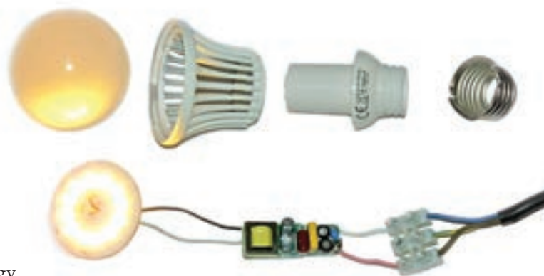
A disassembled LED lamp showing the emitting material, dispersive cover, driver circuit board and Edison screw. Dmitry G./Wikimedia Commons
