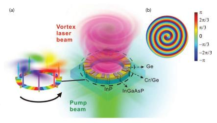
(a) Schematic of OAM microlaser. (b) Simulated phase distribution of laser radiation. The electric-field phase changes by  $2\pi$  upon one full circle around the center of the vortex. The phase is continuous everywhere except for the center of the emission path, presenting a topological phase singularity point at the beam axis.
