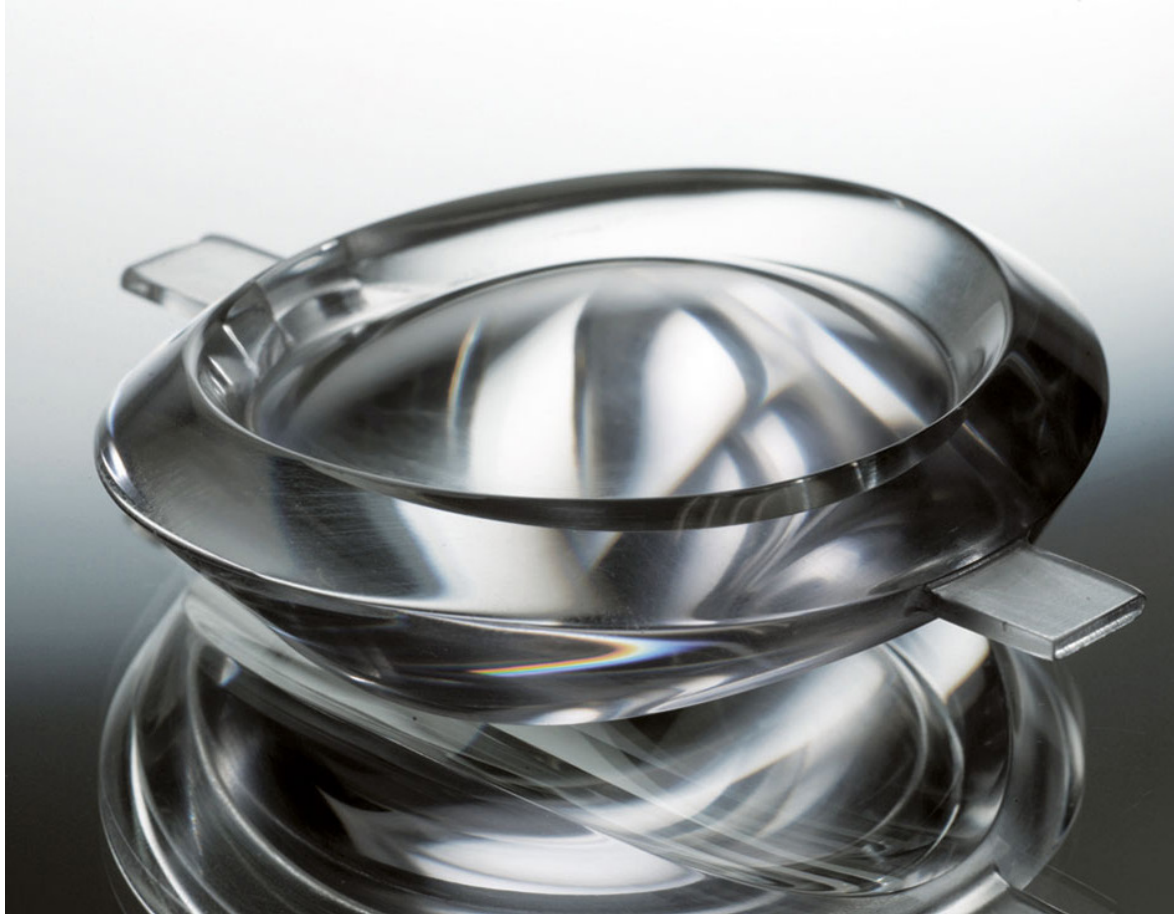
Compact freeform lens for a fog light. Fraunhofer Institute for Laser Technology ILT, Aachen/Germany
