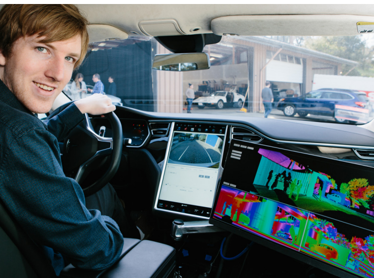
Left: Luminar co-founder Austin Russell in car with lidar images. Right: Luminar lidar records a point cloud image its surroundings; colors convey information such as distance to the objects observed. Images courtesy of Luminar
