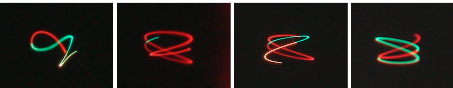
In an optical-trap display, a light-scattering particle confined in a nearly invisible optical trap is dragged through space to create a 3-D image.
