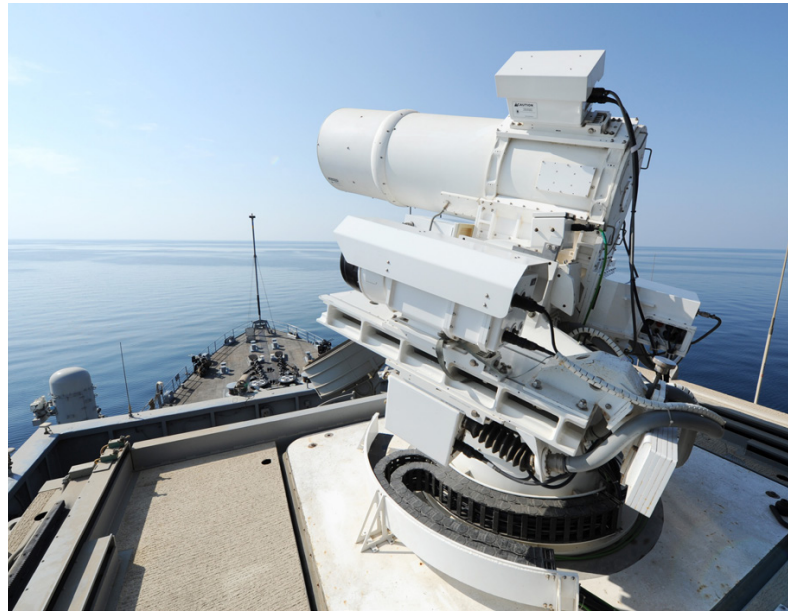
The U.S. Navy's fiber-based Laser Weapon System (LaWS) was tested in 2014 aboard the USS Ponce in the Persian Gulf. U.S. Navy photo
