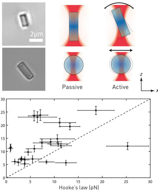
Top, left: Zeolite-L crystals observed from the side. Top, right: Schematic side view of cylinder and sphere in optical traps. Passive: resting probes; active: probes driven through viscous media, causing displacement and torque (visible as rotation of the cylinder). Bottom: Comparison of direct force sensing with Hooke's law. Direct forces are above the unity line, indicating the presence of rotation.
