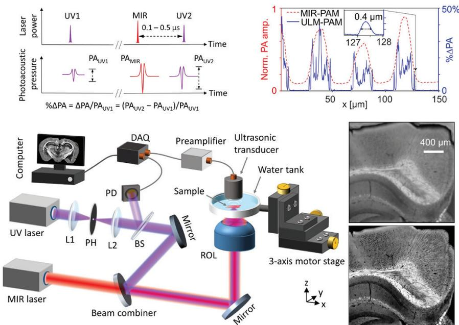
Top left: Principle of ULM-PAM. Bottom left: Schematic of the experimental setup. BS, beam splitter; DAQ, data acquisition unit; L1, L2, lenses; PH, pinhole; ROL, reflective objective lens. Top right: Amplitude profiles of conventional MIR-PAM (red) and ULM-PAM (blue) images across a pattern of vertically aligned carbon nanotubes. Bottom right: MIR-PAM (upper image) and ULM-PAM (lower image) image of myelin in a mouse brain slice with a 300-μm thickness. [Adapted from reference 5.]
