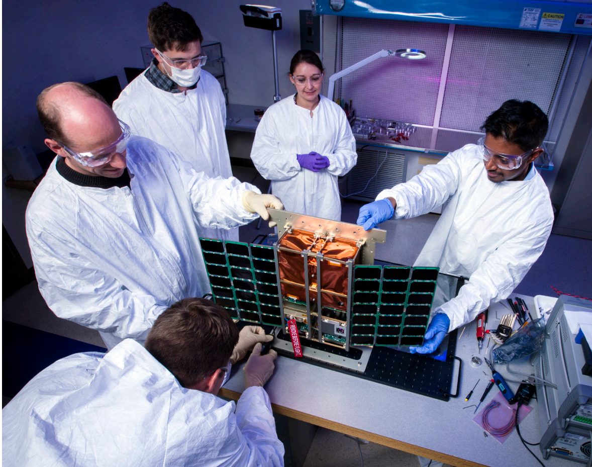
Technologists integrate a Goddard-developed instrument into Lawrence Livermore National Laboratory's (LLNL) CubeSat bus. Lawrence Livermore National Laboratory
