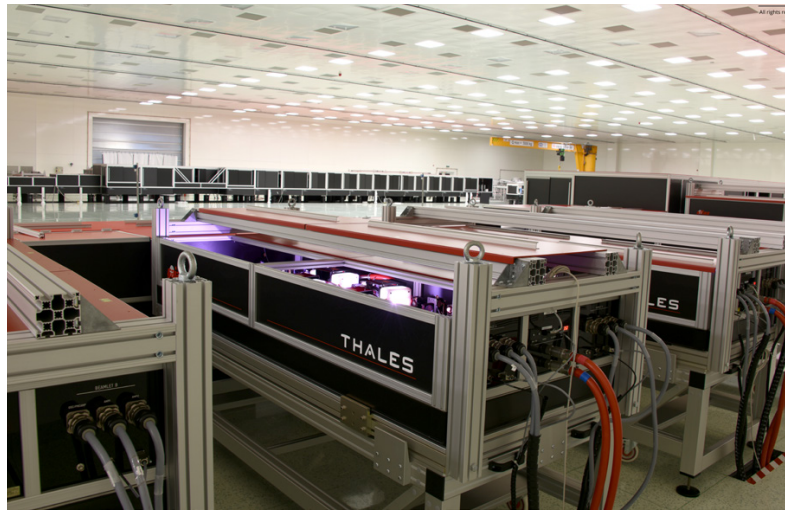
The laser arms built for ELI-NP by the French company Thales are, at present, the most powerful operational lasers in the world. Courtesy of ELI-NP
