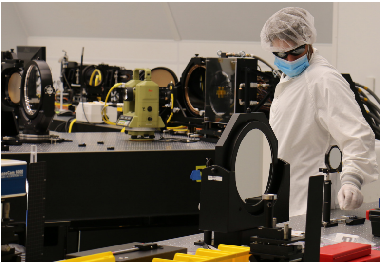
A scientist works inside DKIST's Coudé lab. The physics lab, which weighs 150 tons, rotates to position five scientific cameras as the telescope tracks the sun across the sky. Mirrors, beam splitters and filters split the light so each camera receives a beam.
