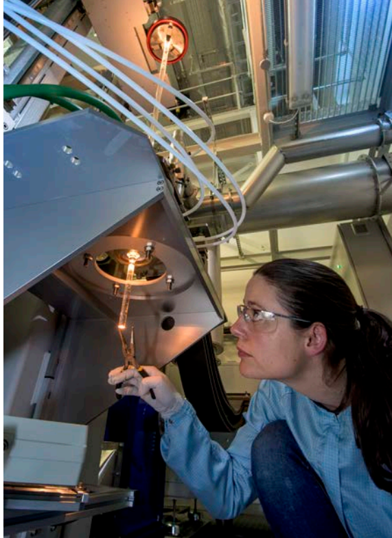
Left: Researcher Natalie Wheeler drawing optical fiber. Right: Creating hollow-core fiber typically involves the drawing of a preform, including capillary tubes and spacing elements stacked within a 20-to-30-mm-diameter tube, into a cane a few mm in diameter. The cane is then packaged in a thicker jacket tube to construct a second preform that is drawn into the final fiber in a fiber drawing tower. During the draw, an inert gas is pumped into the core and capillary regions to control the fiber geometry. University of Southampton / G.T. Jaison et al., Opt. Express 27 , 20567 (2019); doi: 10.1364/OE.27.020567
