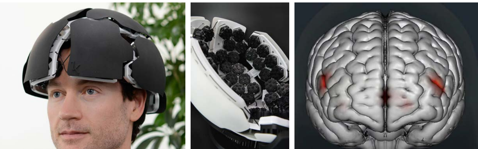
Kernel CEO Bryan Johnson (left), Kernel Flow headwear (center) and activation map from fNIRS, showing activation for a working memory task on a single participant's fifth day of a 15-day study (right).
