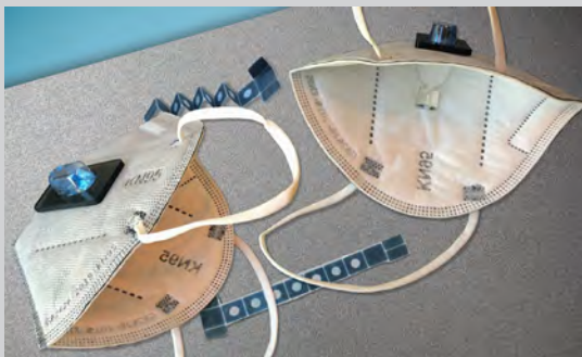
Prototype of the Harvard–MIT team’s facemask-based COVID detection system.
