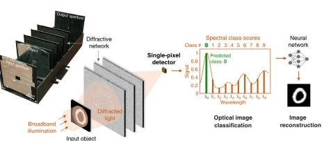
A diffractive optical network encodes the spatial information of objects into the spectrum of the diffracted light, to classify input objects and reconstruct their images using the output spectrum detected through a single-pixel.
