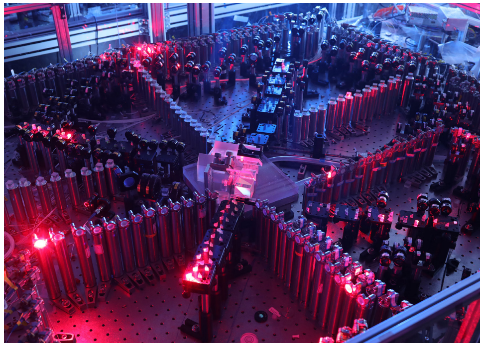
The interferometer part of the experimental setup. The photonic device is realized by sending 50 single-mode squeezed states into a 100-mode interferometer, and then sampling from the output distribution using 100 single-photon detectors.
