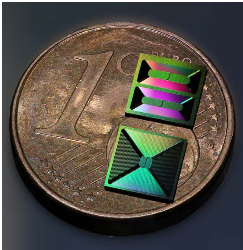
Photograph showing \text{Si}_3\text{N}_4 photonic chips containing two meter-long (upper chip) and one 1.4-meter-long (lower chip) spiral waveguides.
