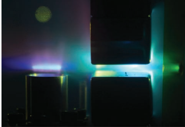
Laser wakefield accelerator research using the Gemini laser at the UK's Rutherford Appleton lab. The purple/pink column on the left is the plasma, about 2 cm long. The blue light to the right, emitted by the interaction, is reflected off one of the magnets used to steer the electron beam.
