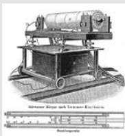
Early apparatus for measuring spectrum of blackbody radiation
