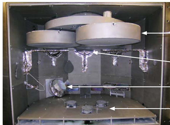
Exterior (top) and interior (bottom) views of the 2.3x2.3x1.8-m large-optics vacuum coating chamber at Sandia National Laboratories. The chamber, in a Class 100 cleanroom, is equipped for electron-beam evaporation of coating materials, with or without ion-assisted deposition provided by an RF ion source. The planetary rotational fixtures can accommodate optical substrates of dimension up to 1.2 m, with masking to provide for thickness uniformity of coating layers on large substrates.
