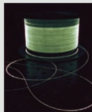
Erbium-doped optical fiber
