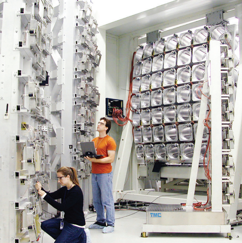
The final mirror array inside the Nike laser facility at the US Naval Research Laboratory.
