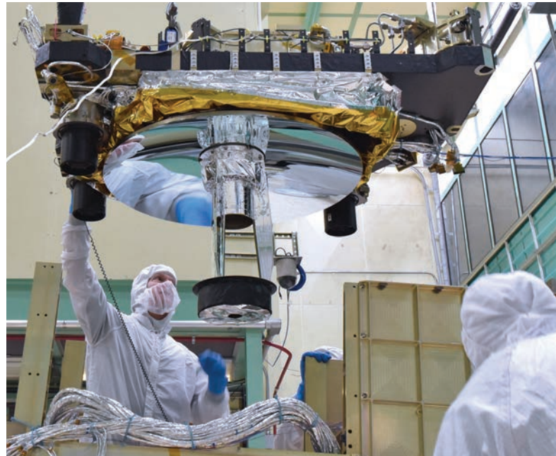
Engineers and technicians integrate the Global Ecosystem Dynamics Investigation instrument's optical bench and box structure.
