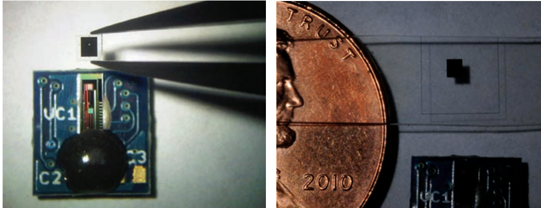
Simple optical preprocessing with pinhole diffraction provides a 180-degree field of view. The printed pinhole (shown between forceps) is mounted on a Centeye 125-mg TinyTam 16x16 sensor. A US penny is provided for scale. Courtesy of Centeye
