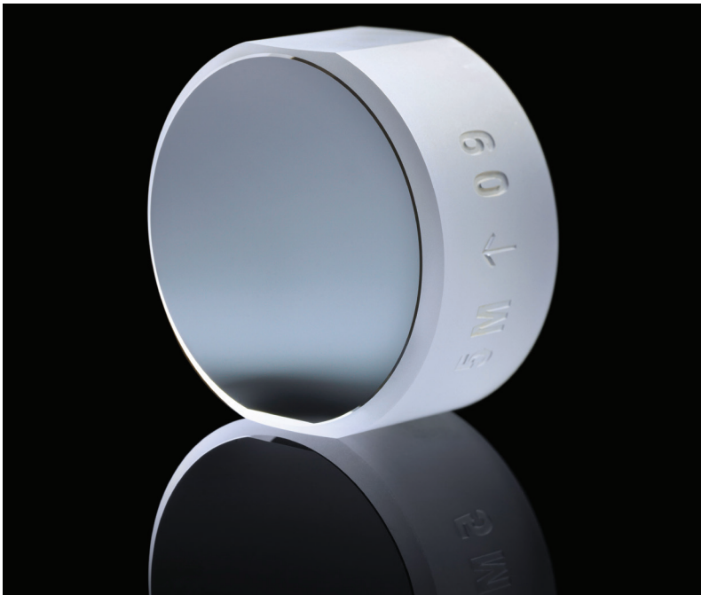
Prototype semiconductor supermirror (GaAs/AlGaAs direct-bonded to fused silica).
