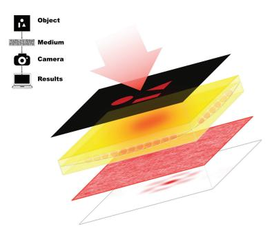
An object hidden behind an opaque layer is illuminated by a spatially incoherent narrowband light source. The object light passes through the scattering medium to the camera sensor, forming a random speckle pattern. Performing the cross-correlation product of the measured speckle patterns taken at different times makes it possible to track moving objects.
