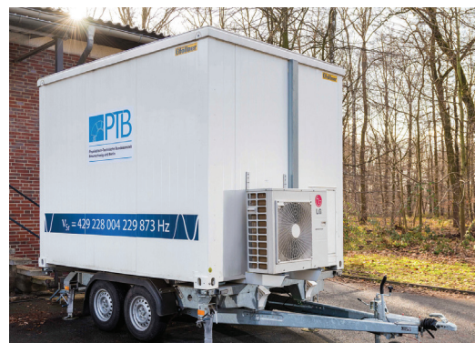
A transportable strontium-87 lattice clock developed by researchers at the Physikalisch-Technische Bundesanstalt, Germany, and its trailer seen from the outside.
