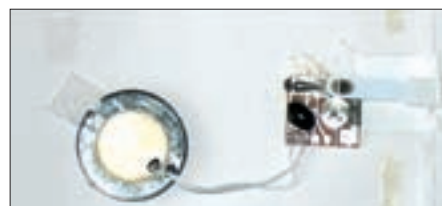
Top: THz transmission image of a battery, circuit and speaker — which, together, form a device that is used in a musical greeting card to play music when the card is opened (bottom).
