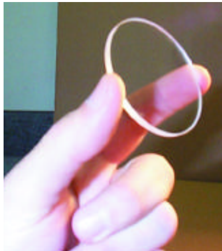
Figure 3. A typical optical window with a high aspect ratio. (Photo courtesy of QED Technologies.)
