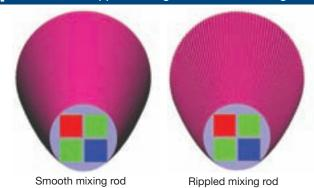
The taper provides an angle-to-area transformation, changing the full hemisphere Lambertian output of the LEDs into a distribution that fills a smaller cone angle (30 degree half cone angle in this example).
