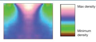
The extractor density is lower near the LEDs and varies across the light guide to achieve the desired uniform output.
