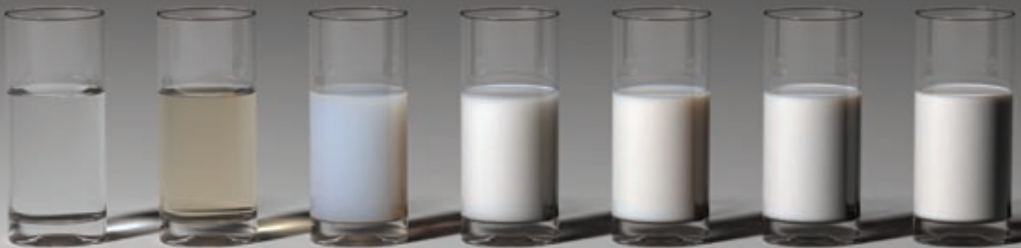
Photorendered milk and its components. Jensen and colleagues computed the optical properties of the solutions using Lorenz-Mie theory. From left to right, the glasses contain water, water and riboflavin, water and protein, water and fat, skim milk, reduced-fat milk and whole milk.
