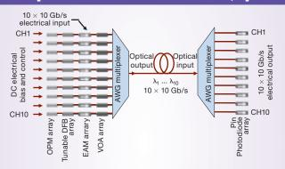
In this block diagram, the TX chip consists of 10 tunable lasers, 10  $\times$  10 Gb/s electro-absorption modulators (EAMs), and 10 variable optical attenuators (VOAs), all coupled to an arrayed-waveguide grating (AWG) multiplexer. In addition, 10 optical power monitors (OPMs) are also integrated monolithically on the transmitter chip. The RX chip consists of 10  $\times$  10 Gb/s high-speed photodetectors coupled to an AWG demultiplexer.
