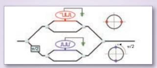
Nested Mach-Zehnder modulator used in DQPSK optical data transmission systems. Light can be split into four equal paths and modulated in two different data streams in this example. To achieve phase quadrature, one branch needs to be rotated a quarter-turn (or  $\pi/2$ ).
