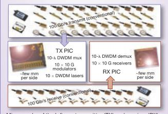
Micrographs of the Infinera transmitter (TX) and receiver (RX) PICs (a few mm on a side), compared with all the discrete components they replace (several cm per component).
