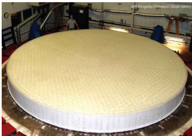
The first GMT segment rests on the furnace hearth after a successful casting. The honeycomb sandwich mirror is a single piece of glass containing 1,700 hexagonal cavities. The ceramic fiber mold that forms the cavities is still inside the mirror at this point, but it is washed out in a later operation.
