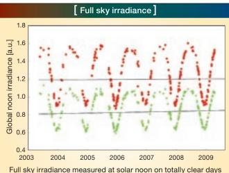
Full sky irradiance measured at solar noon on totally clear days by a Radio Shack Sun and Sky Monitoring Station. The data show no noticeable drift during the six years the instrument has been used at the author's South Texas site.
