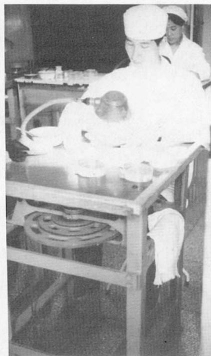
Fine hand polishing of a multifaceted scanner used in thermal imaging systems done on a treadle wheel at the North China Optical Factory, Beijing.
