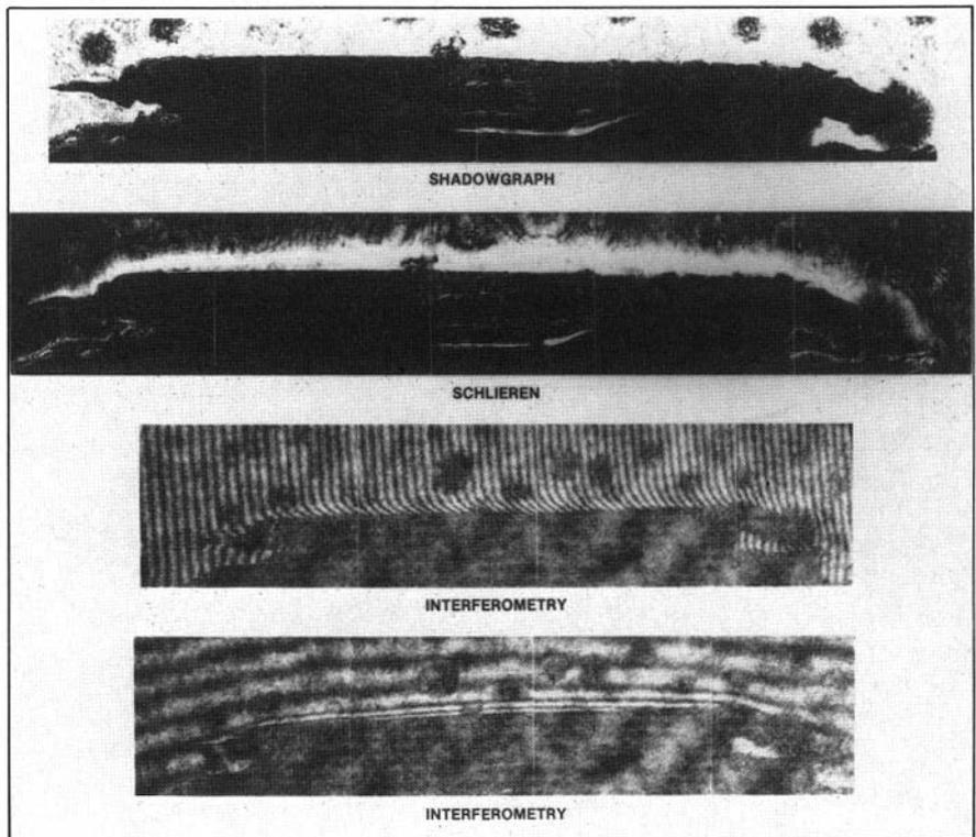
*Results from FES hardware check-out. Test holograms from the FES were used to generate shadowgraph, schlieren, and interferometric images of a growing TGS crystal. All images were made from the same hologram. The main virtue of holography for this experiment is that it allows such techniques to be applied as required in the laboratory after the flight, rather than trying to perform them during the mission. (Holographic reconstruction performed by W. K. Witherow, MSFC)*
