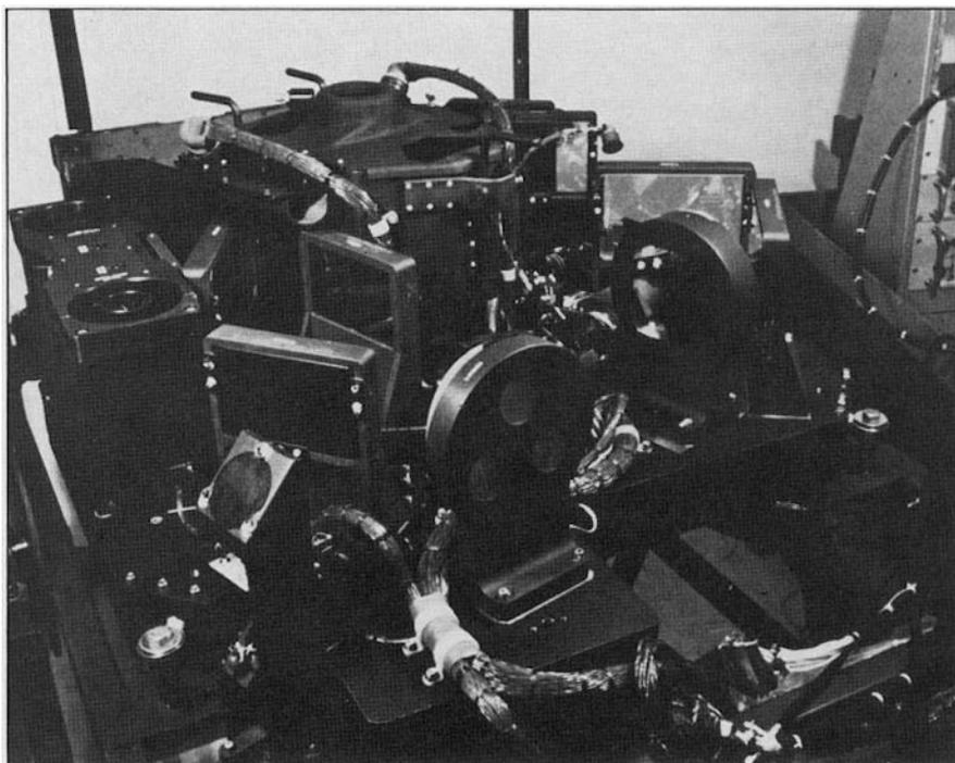
*FES flight optical system. This photograph shows the actual FES flight holographic schlieren system.*
