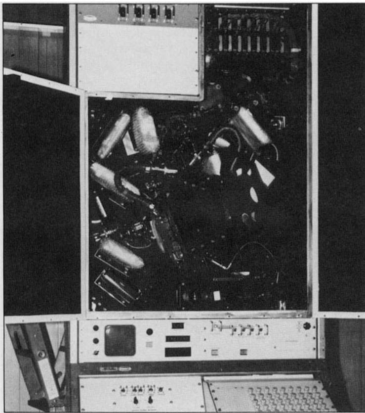
**FES optics in rack-assembly.** The FES optical system is shown mounted in the Spacelab rack. The FES control panel includes a TV screen which allows the schlieren image of the growing TGS crystal to be viewed by the payload specialist during flight. Controls are also available to allow manipulation of the schlieren knife edge.
