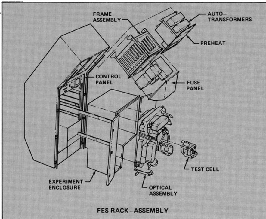
**FES rack-assembly.** This schematic shows how the FES flight optical system and test cell mount into a standard Spacelab rack. The locations of support electronics and controls are also shown.
