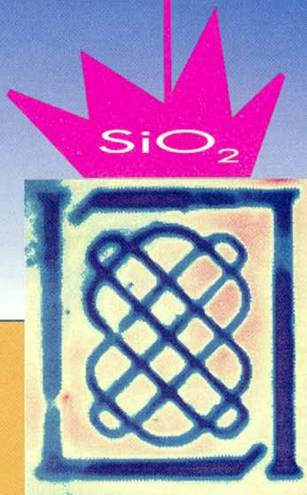
Figure 2. Top view of a sample of fused silica, as seen (in pseudocolors) with a phase measuring interferometer (PMI), following irradiation with a 193 nm excimer laser. The pattern is imprinted in the 1 cm-thick material by laser induced compaction (dark areas) of ~100 nm. The irradiation was performed through a prepatterned Cr-on-quartz mask. The pattern represents Lincoln Laboratory's logo; it is ~4.034.5 mm in size, the thin lines being ~150 \mu\text{m} wide. This sample seems unaltered by the laser radiation, except when viewed through the PMI.
