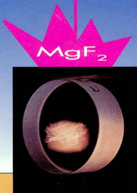
Figure 1. Sample of \text{MgF}_2 fluorescing under exposure to 193 nm excimer radiation. The sample has a large number of crystalline grain boundaries. These did not initially fluoresce differently from the rest of the sample, but after ~200,000 pulses at 100 \text{ mJ cm}^{-2}/\text{pulse} they suddenly became much brighter, as seen in the figure. The reason for this behavior is not well understood, although one may conjecture that fluorescing crystalline defects are preferentially formed by the laser at the grain boundaries.
