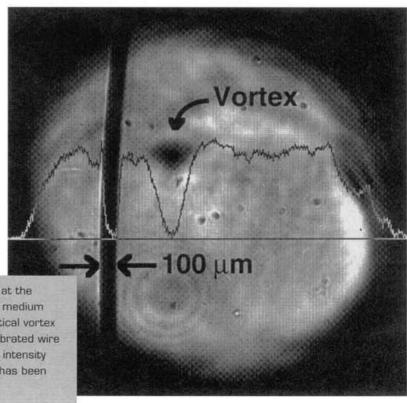
Cross-sectional intensity profile at the output face of a self-defocusing medium showing the dark core of an optical vortex soliton. The dark stripe is a calibrated wire 100 µm wide. A line plot of the intensity profile through the vortex core has been superimposed on the image.
