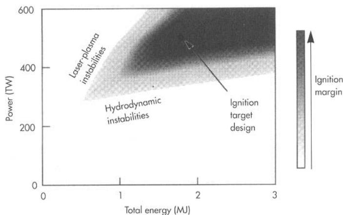
**Figure 4.** The National Ignition Facility's Indirect-drive target design meets the criteria of acceptable target performance for hydrodynamic and laser-plasma instabilities.
