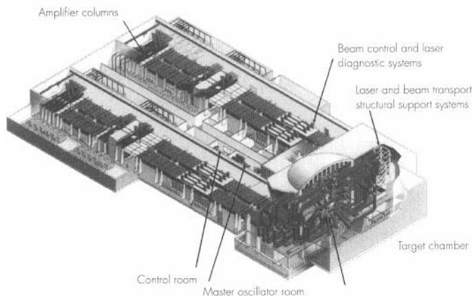
**Figure 5.** Schematic diagram of the 192-beam National Ignition Facility.
