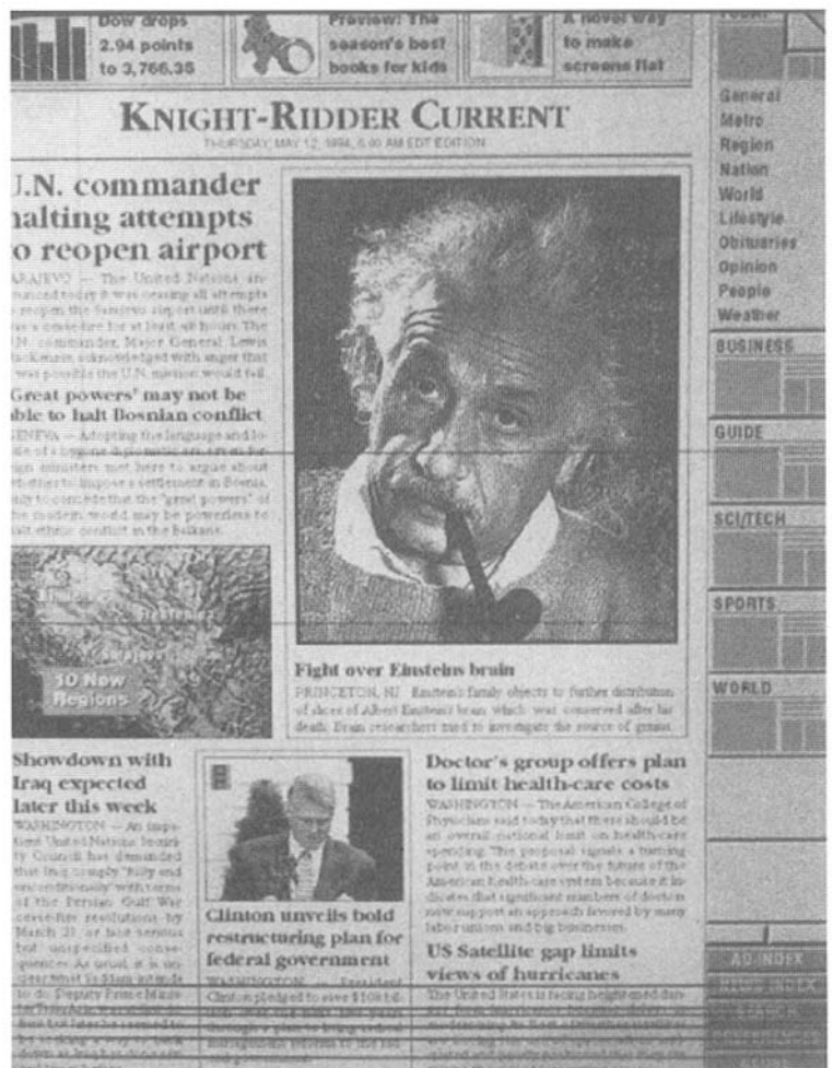
Figure 4. Surface stabilized cholesteric display 20 produced at the Liquid Crystal Institute. Electronic tablets such as this may become the newspaper of the future.
