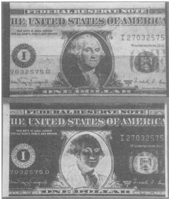
Figure 3. Laser-written image of a dollar bill in a liquid crystal cell, viewed between crossed polarizers, using a photosensitive alignment layer. The negative image is produced by rotating the analyzer 90°. The resolution is 600 dpi. [Produced by W. Gibbons (Hercules Inc.), T. Kosa and P. Palffy-Muhoray (Liquid Crystal Institute, KSU).]
