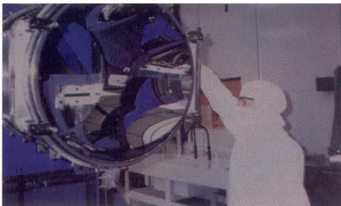
Figure 3. The smallest AXAF paraboloid is shown in its handling fixture after being coated with iridium at Optical Coating Laboratories Inc.
