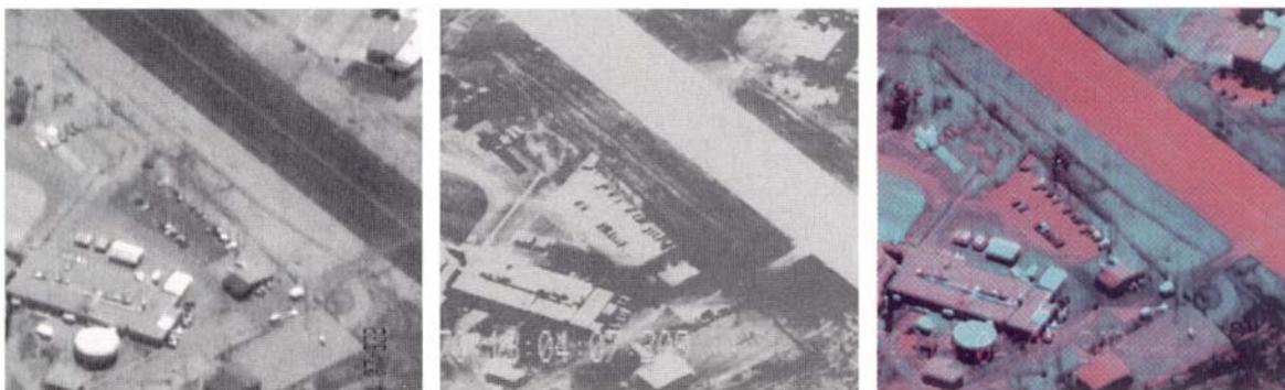
**Figure 7.** A daytime image taken from an aircraft flying over an industrial site in a desert setting using a TV camera and an LWIR FLIR. All the information from both bands is seen clearly in the composite color image. Color aids in clearly delineating buildings, parking areas, vegetation, and barren soil.
