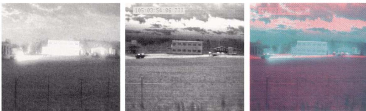
**Figure 6.** A nighttime dualband image taken with a low-light level camera (responsive in both the visible- and NIR-bands) and an uncooled LWIR camera. In the single-band low-light level image, there is some blooming and a number of dark areas. In the LWIR image, these same areas have better contrast. The composite color image shows that the imagery from both bands can be combined with essentially no loss of information in a clear and intuitive color image.
