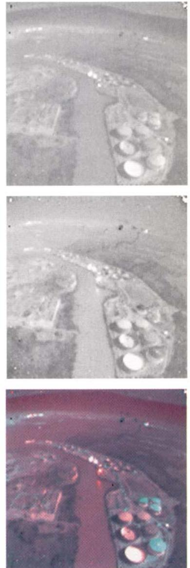
**Figure 5.** An airborne image taken with a dualband MWIR/MWIR sensor of an industrial plant on a river. The exhaust flume is very saturated in the red band and the storage tank in the near-field is bright cyan as a result of strong solar reflections.
