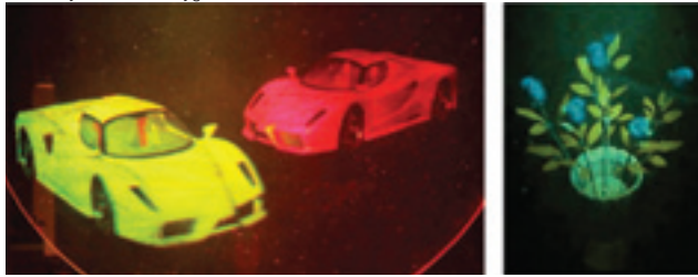
3-D updatable holograms recorded on photorefractive polymers. (Left) A 17-in. red and green display (and all combinations of the two colors) and (right) an 8-in. blue hologram.
