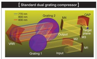
Optical 3-D layout of a compressor with the off-axis parabola (OAP) used to focus the beam. M1 to M4 are folding mirrors and VRR is the vertical retro reflector.
