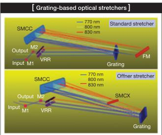
Optical 3-D layout and beam propagation for two optical stretchers using Zemax. M1, M2 and FM are folding mirrors, SMCC is a concave spherical (or parabolic) mirror, SMCX is a convex spherical mirror and VRR is a vertical retro reflector. These layouts are necessary for accurate dispersion calculations.
