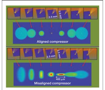
(Top) Final focus images obtained with Zemax ray tracing of an ultrafast laser. A 2.5 mm<sup>2</sup> square detector screen is scanned across the focus produced by an F/3.6 off-axis parabola. The compressor is perfectly aligned. The spot is diffraction-limited and pictured in the middle as a dot. (Bottom) Similar images appear if the compressor is misaligned by a 0.05 degree rotation of the 2<sup>nd</sup> grating in the plane of dispersion.
