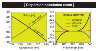
(Left) The delay introduced by one compressor and three stretchers. The stretcher delay curves appear as one because there are extremely small differences between them. (Right) The residual delay from summing the compressor and the stretcher delay curves. The Offner stretcher is almost exactly opposite of the compressor because the residual delay is almost zero from 760 nm to 840 nm.
